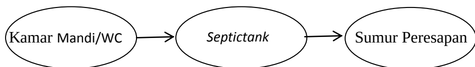
Gambar 2.5 Alur Sanitasi Septictank
